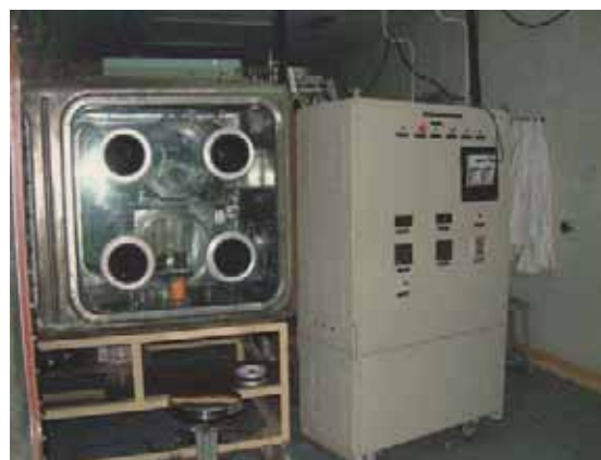
Fig.1: Microwave Heating System adapted inside Glove-Box
