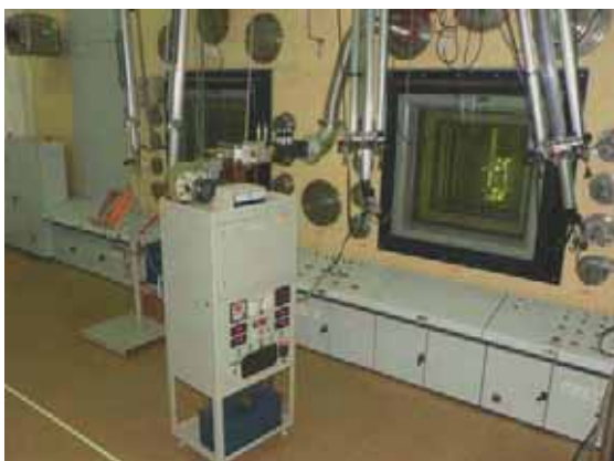
Fig. 2: Microwave Heating System adapted inside Hot-Cell
