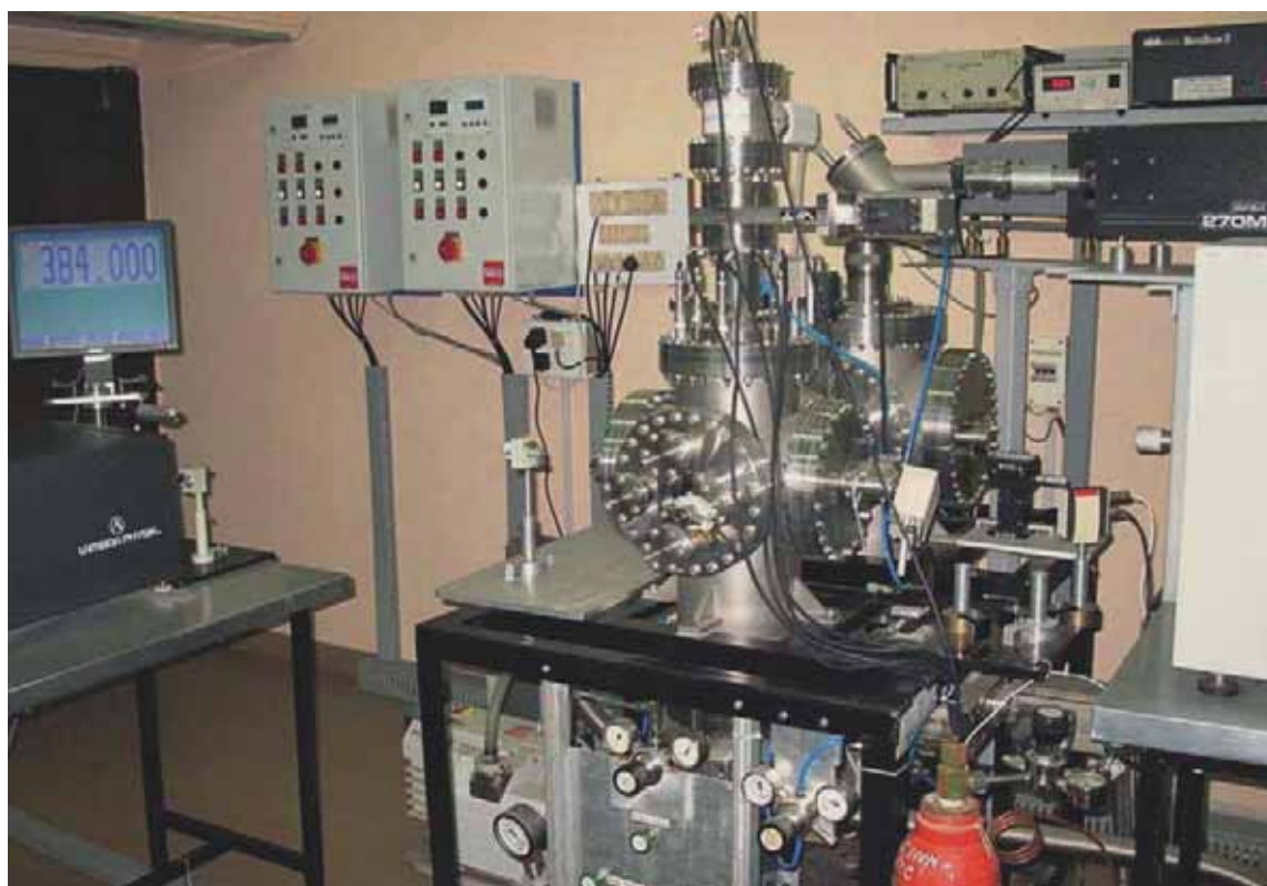
Fig. 2: Photograph of the supersonic molecular beam setup.
